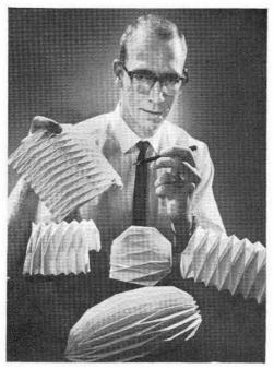
DEAN GLADOW displays small folded paper models of types of collapsible structures possible with his construction method. Size is no limitation. With proper materials, folding structures as large as a football stadium could be built.
